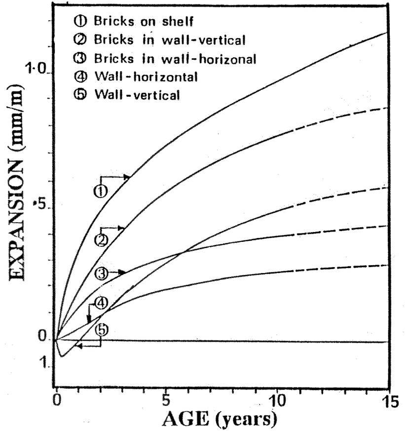
Figure 2. Expansion v Time: Unrestrained wall
