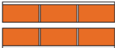
Figure 9. Rendered cavity brickwork, 110 mm clay bricks
